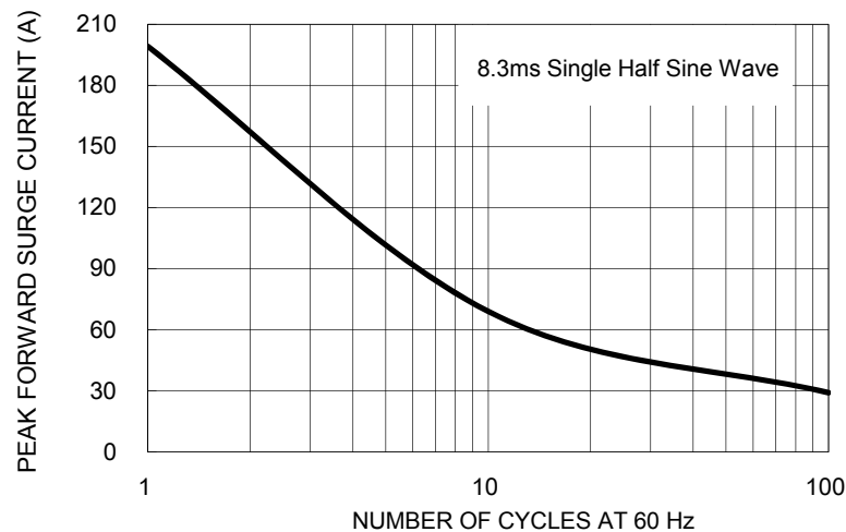
FIG.3-MAXIMUM NON-REPETITIVE PEAK FORWARD SURGE CURRENT
